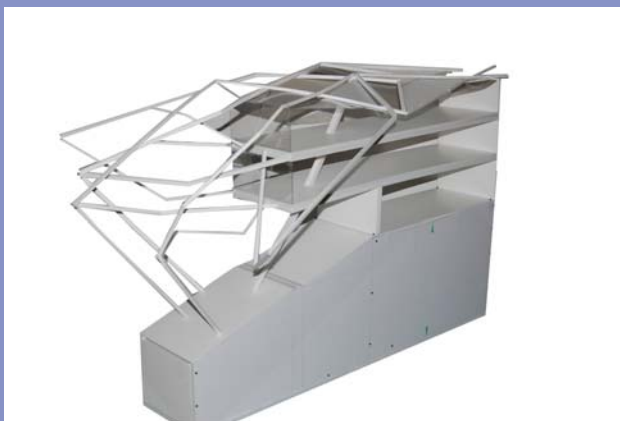
Study of the roof construction
